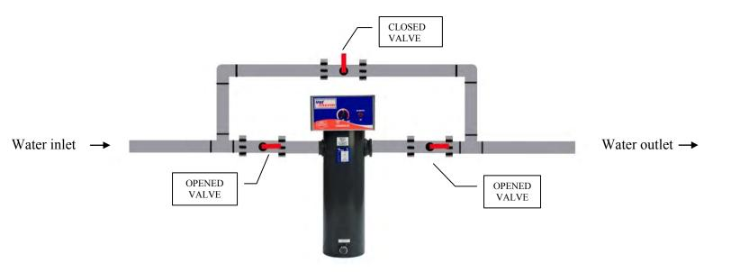
It is recommended to install a by-pass on the plumbing of the water heater
