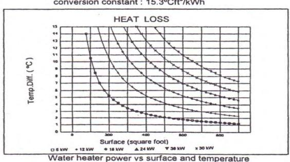
Rule of thumb: for each KW per 1000 gallons of water, you can add 1 F° of temperature elevation an hour.
