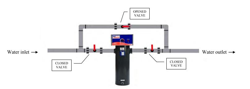
1 is recommended to isolate your water heater on the water by pass when you do your shock treatment at the opening of you pool not to damage the component.
